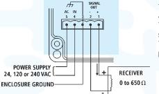
Terminals 1 and 2 are 4-20 mA current output. Terminal 3 is the enclosure ground. Terminals 4 and 5 are AC power input.
