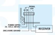
Terminals 1 and 2 are DC voltage output. Terminal 3 is ground. Terminals 4 and 5 are AC power input.
