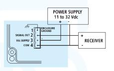
Terminal 1 is enclosure ground. Terminal 2 is positive signal voltage. Terminal 3 is positive supply voltage. Terminal 4 is common to both the DC power supply and the output signal.
